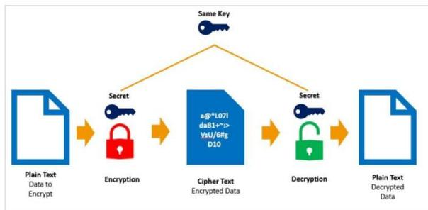
Fig Encryption Process
