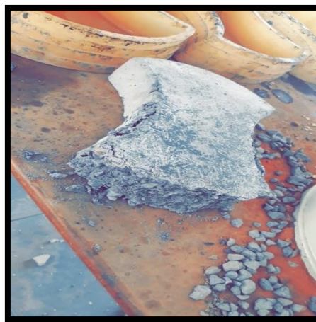
compressive strength test
