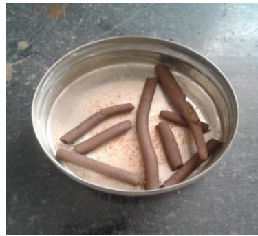
Fig : D Plastic limit (Soil Rolled in 3mm thread)
