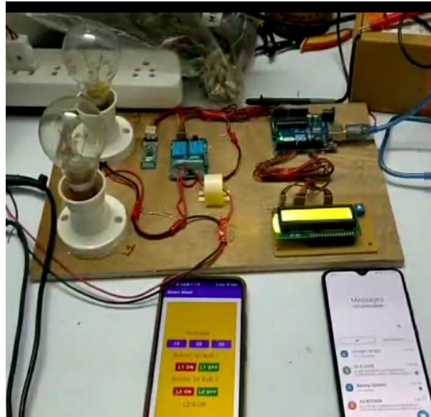
FIG VII: The internal circuitry of Smart Energy Meter
