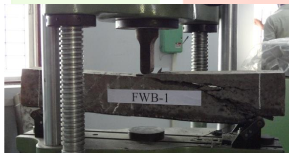
Figure 4.2 Failure mode of FWB-1
