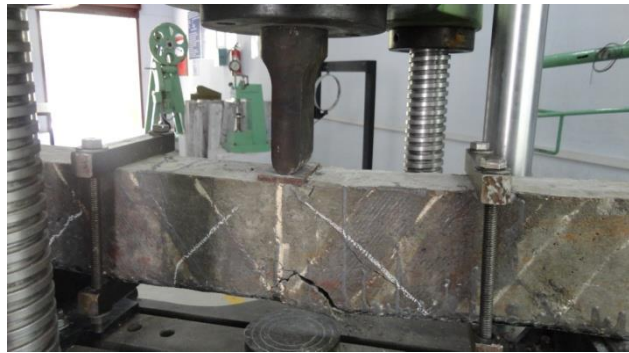
Figure 4.4 Failure mode of FWB-EL-2
