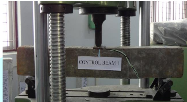
Figure 4.1 Failure mode of Control Beam 1
