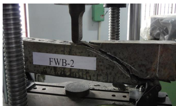
Figure 4.3 Failure mode of FWB-2
