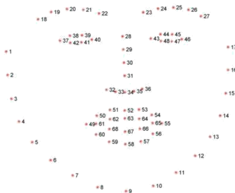
Figure 2: Visualizing the 68-point facial landmark coordinates
