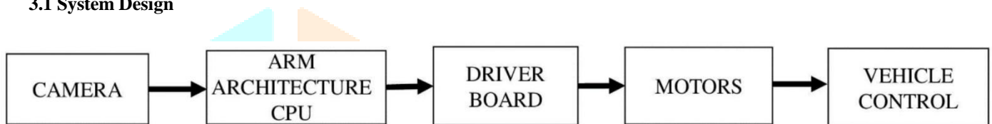
Fig(a) Block diagram of Autonomous Vehicle
