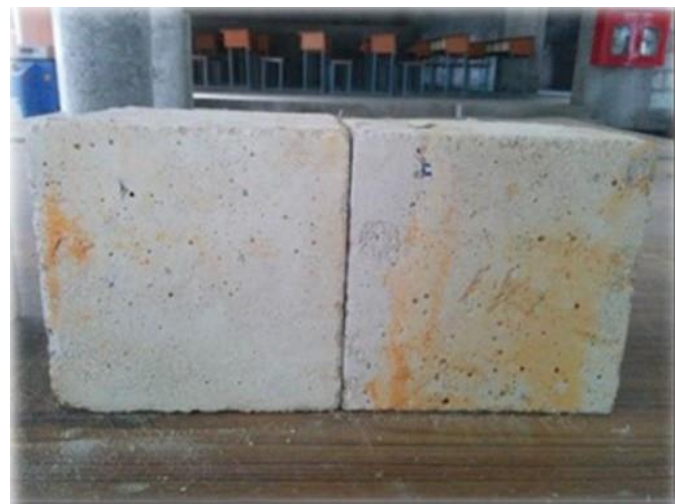
Fig 1: Hydrochloric Acid Attack on Concrete
