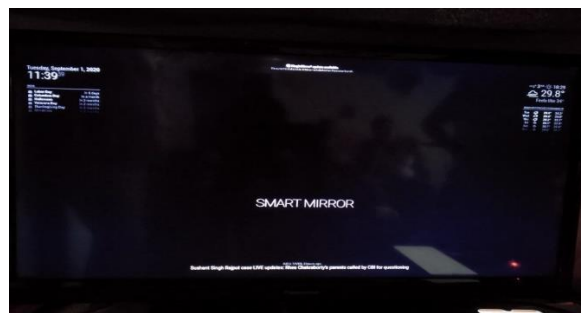
Fig.7 Main Display for Smart Mirror System Smart mirror displays the project title, temperature, time on plasma display. This display is made of plasma display which is preferred over LCD and LED for our application.
