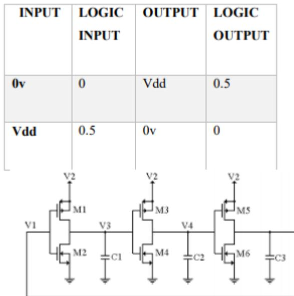
Fig 5 Schematic of three cascaded inverters
