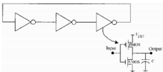
Fig 2. Three stage ring oscillator with internal circuit.
