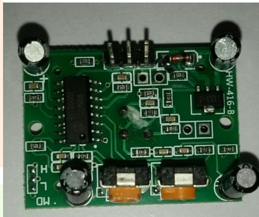
Figure 3: Passive Infra-Red (PIR) Sensor
