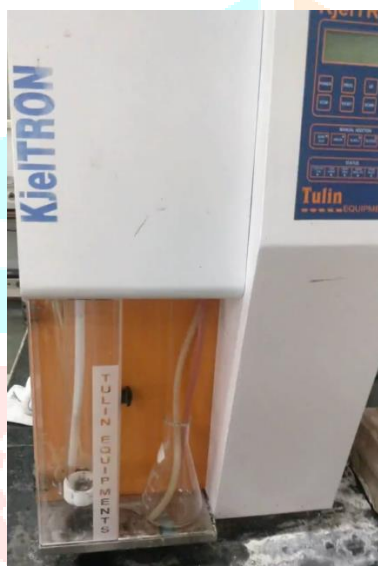
Figure 15: KjelTRON™ - Rapid Automatic Nitrogen Estimation System (Nitrogen Analyser) – Distillation Unit
