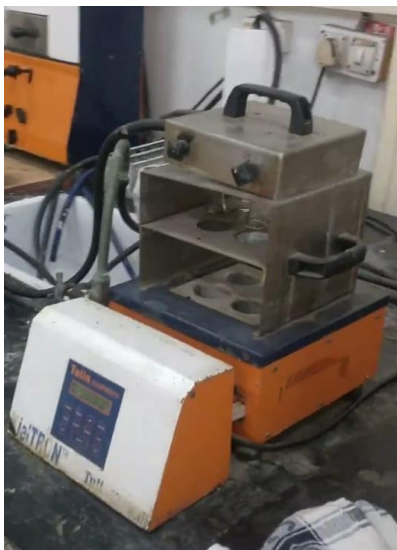
Figure 14: KjelTRON™ - Rapid Automatic Nitrogen Estimation System (Nitrogen Analyser) – Digestion Unit
