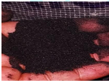
Figure Error! No text of specified style in document..3 Rice Husk Ash
