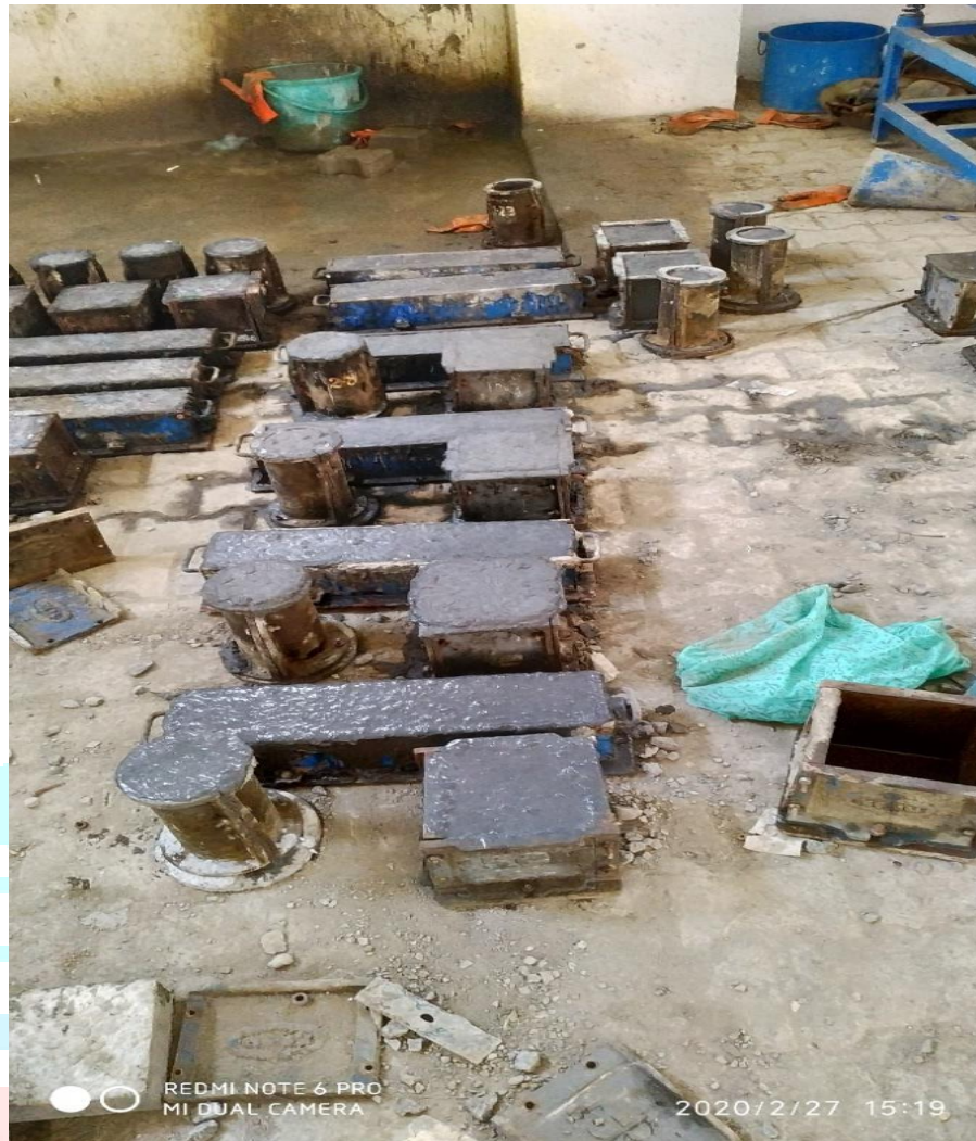
Figure Error! No text of specified style in document..8 Casting of ECC
