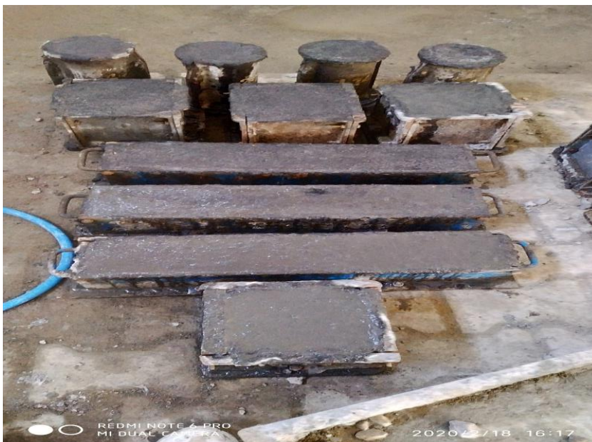
Figure Error! No text of specified style in document..9 Casting of ECC Specimens
