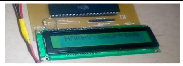
2. When customer scans with RFID tag with the RFID reader, LCD will display no.of items, product cost and the total amount.
