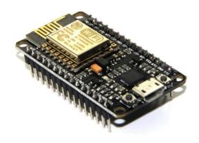
MCU stands for microcomputer and is made up of an integrated circuit chip made of Metal oxide Semiconductor (MOS). It is mainly composed of a microprocessor and peripherals for input and output. It's commonly used in embedded software and other general-purpose software. Microcontrollers can be embedded into any automation and control system. It can be infinitely customizable and sized to fit the circuit.
