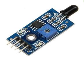
This Flame Sensor can be used to detect fire source or other light sources of the wave length in the range of 760nm - 1100 nm. It is based on the YG1006 sensor which is a high speed and high sensitive NPN silicon phototransistor. Due to its black epoxy, the sensor is sensitive to infrared radiation. Sensor can be a great addition in a fire fighting robot, it can be used as a robot eyes to find the fire source. When the sensor detects flame the Signal LED will light up and the D0 pin goes LOW.
