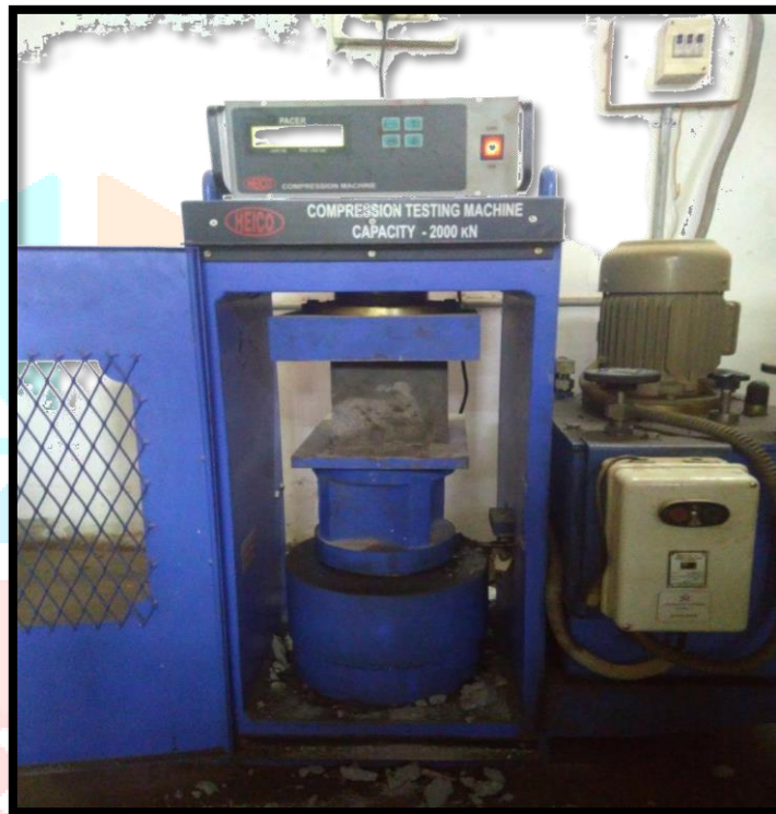
Figure 2- Compressive Strength Test
