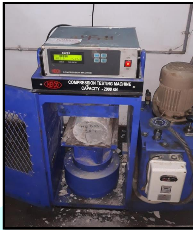
Figure 3- Split Tensile Strength Test
