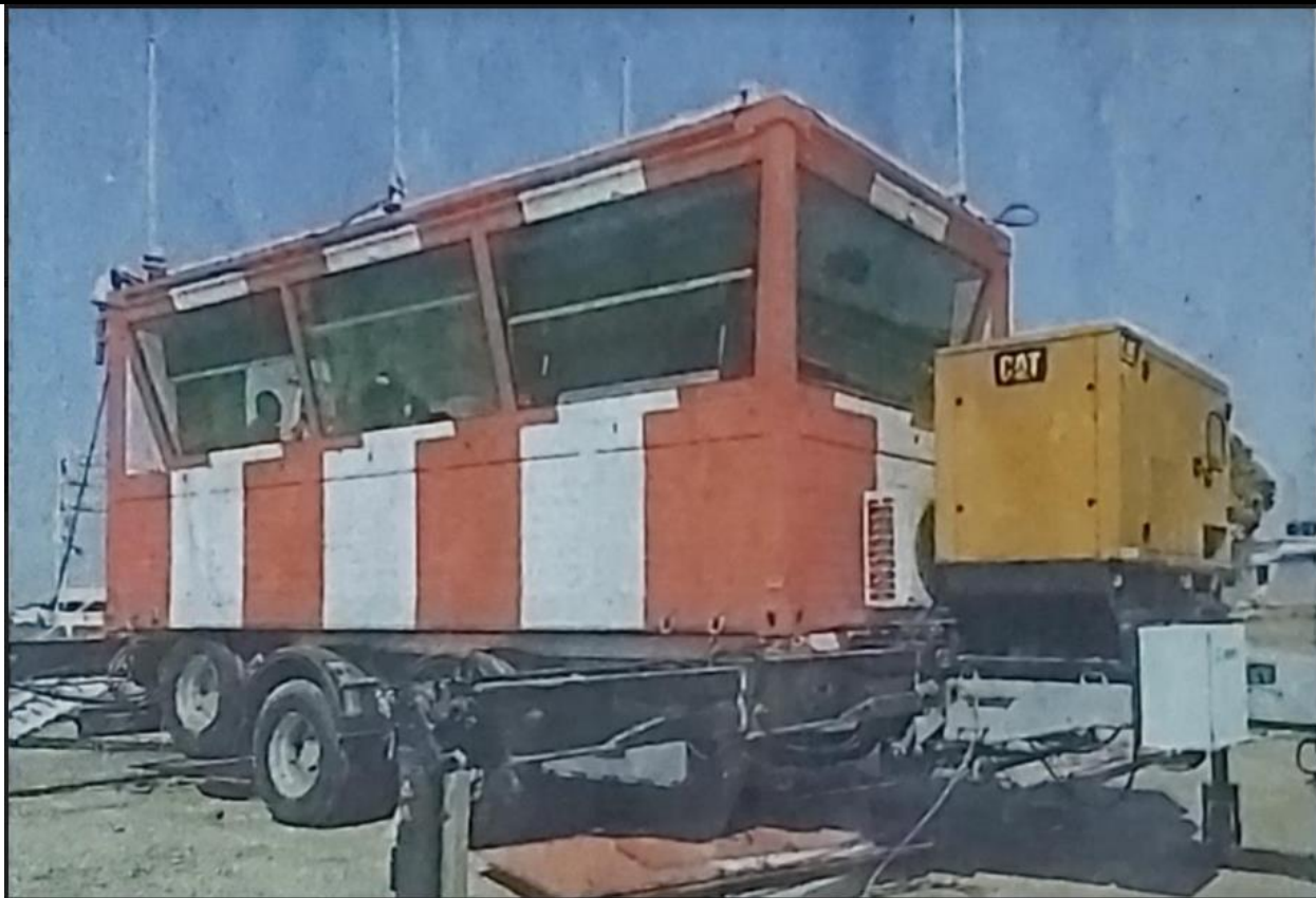
Fig. 3 Imported Air Tower cum navigation system at Bilaspur airport
