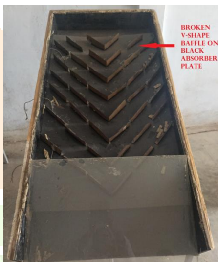
Fig. 3.1 GI black painted broken V-shaped baffle absorber plate
