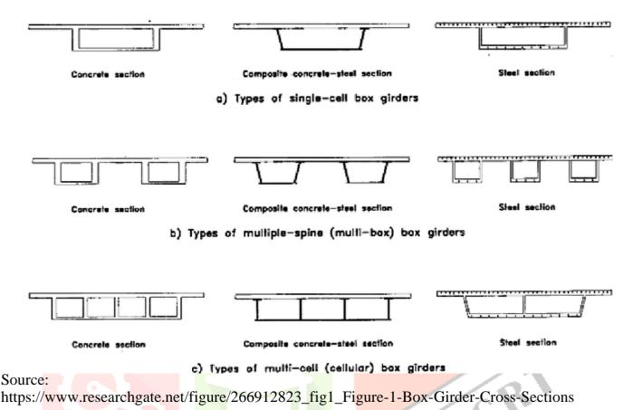
Various girder sections like I-section, T-section, Box girder, hollow core girder, void slab girder, solid slab are used for different span of bridge. Figure 1 illustrates the various types of box girders. Small span bridges are constructed using reinforced cement concrete. As prestressed concrete carries high load over long span, it is used for construction in long span bridge. Span length governs selection of type of section for bridge. For Span length upto 35m.
