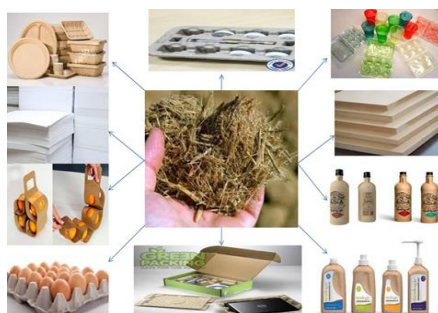
Fig 3 (a) Multiple bagasse products: - tableware, paper, packaging, bottles, MDF board, plastic composite resins
