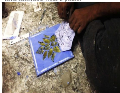
Step 10: The putty and marble powder mixture is applied evenly on the base and then flattened with a planer
