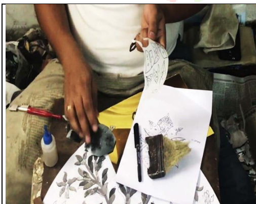
Step 1: A drawing is drawn on a paper and then is traced on an OHP sheet
