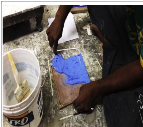
Step 10: The putty and marble powder mixture is applied evenly on the base and then flattened with a planer
