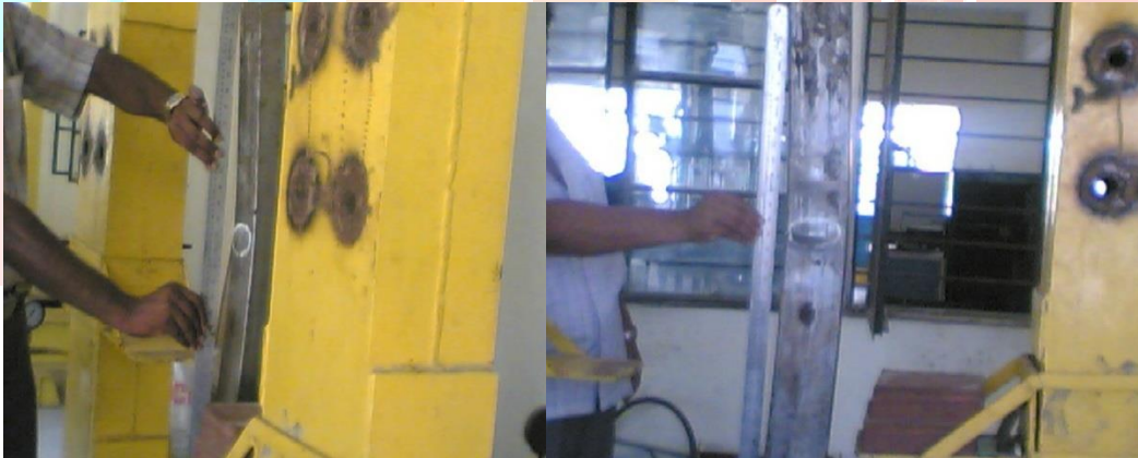
Figure. 5 Double Curvature buckling of columns
