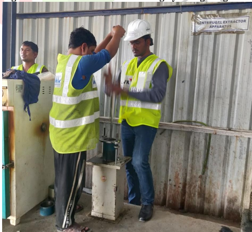
Figure 25 : Tamping the sample to reduce the voides
