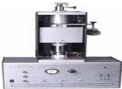
Fig. 3.8 Determination of Thermal Conductivity Using Unitherm™ Model 2022
