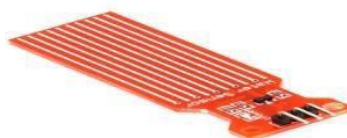
Figure5: Water level indicator
