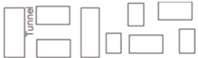
Figure 11 ZIG ZAG PLANNING AVOIDS WIND TUNNEL EFFECT
