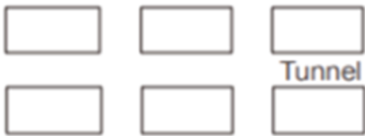
Figure 10 ROW PLANNING CREATES WIND TUNNEL EFFECTS RESULTING IN HIGHER WIND FORCES
