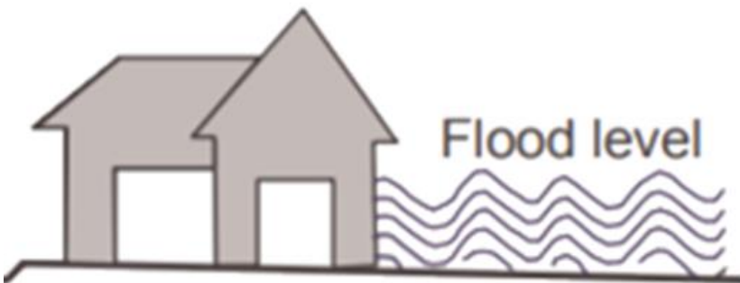
Figure 54 CONSTRUCTION AT LOW LEVEL HAS RISK OF INUNDATION
