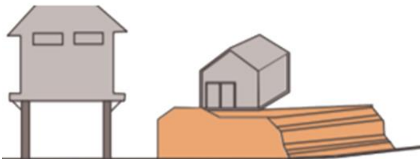
Figure 54 CONSTRUCTION AT LOW LEVEL HAS RISK OF INUNDATION
