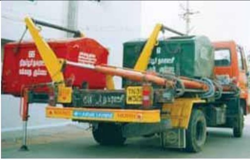
Figure 2 : Skip Truck (Dumper Placer Machines)
