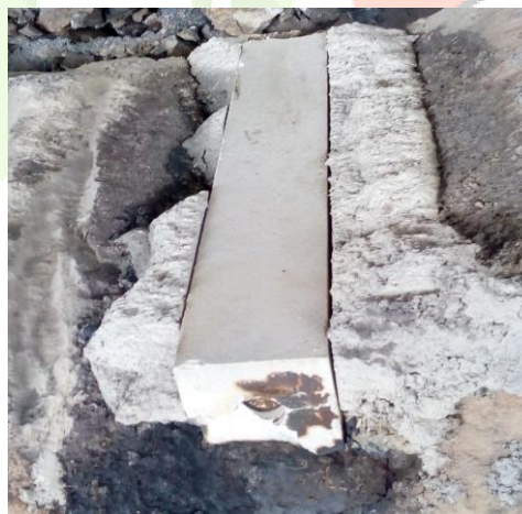
Fig.4 Diffuser at the end of casting
