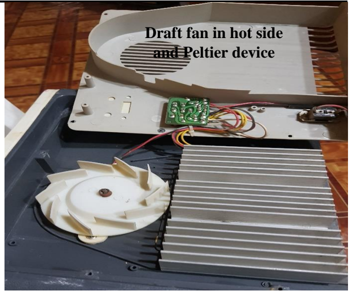
Figure 2: Details of a Draft fan on the hot side
