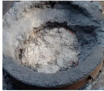
Fig. 7: Flyash LCC in ladle
