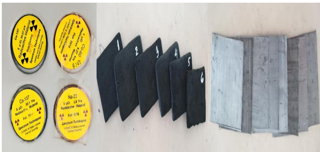
Fig 3. The gamma-ray sources and absorber materials of carbon and lead
