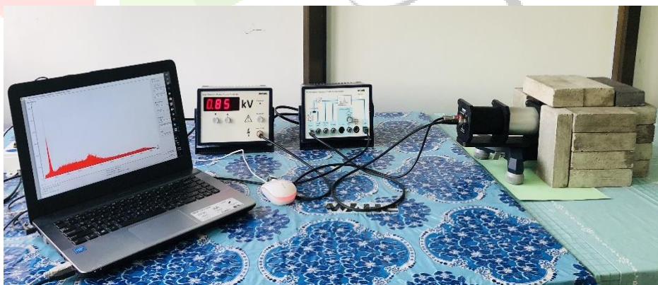
Fig 2. Laboratory equipment for the measurement of gamma radiation spectrum with the scintillation detector
