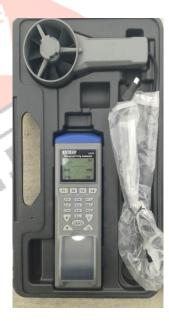
Fig.3 Anemometer + Psychrometer. [8]
