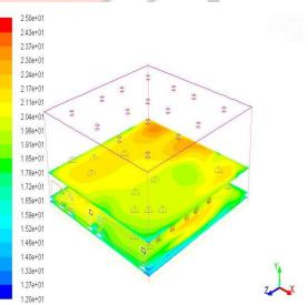
Fig.21: Contours of Relative Humidity for Event Case1.
