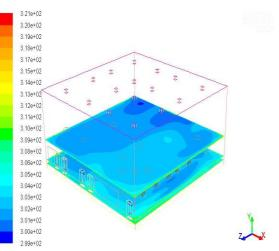
Fig.20: Contours of static Temperature for Event Case1.
