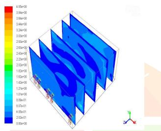
Fig.11: Contours of velocity magnitude for Basic Case1 at z-plane.
