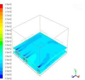
Fig.14: Contours of static Temperature for Basic Case1 at y-plane.
