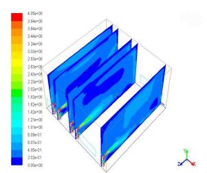
Fig.10: Contours of velocity magnitude for Basic Case1 at x-plane.
