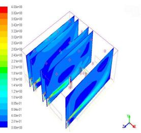
Fig.19: Contours of velocity magnitude for Event Case1.
