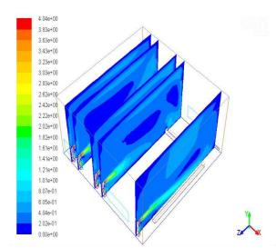
Fig.16: Contours of velocity magnitude for Cooling Case1.
