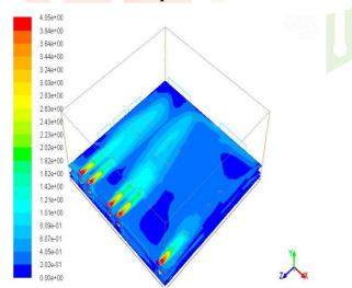
Fig.12: Contours of velocity magnitude for Basic Case1 at y-plane.
