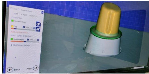
(Fig.7) Designing of the coping
