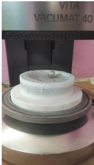
(Fig.11) Ceramic veneering on zirconia copings
