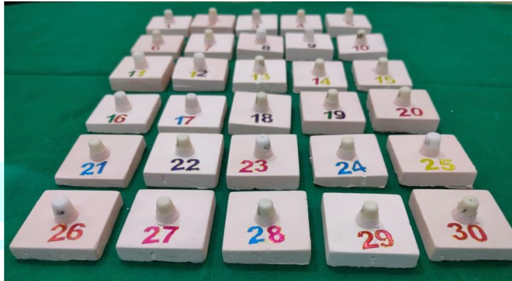
(Fig.8) Milled zirconia copings
