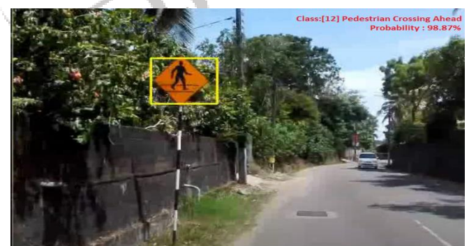
Figure 10: Result of real-time road sign board detection.
