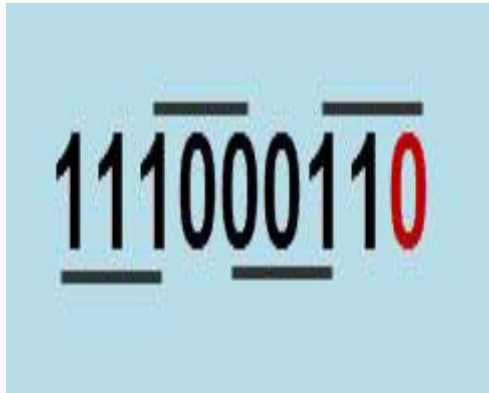
Fig 2. 3-bit pairing for Booth recoding
