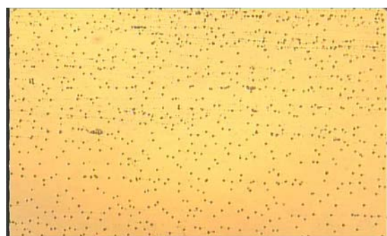
Figure 1: Micrograph of \text{Pb}_{1-x}\text{In}_x\text{Se} ( X=0.2 ) Thin film of thickness 3000\text{ \AA}
