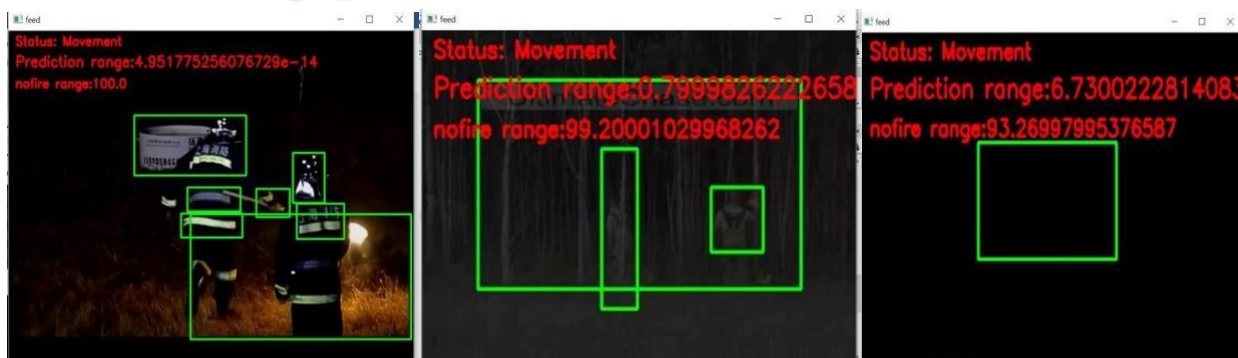
Fig 4: Detection of movement in the video is highlighted by a bounding rectangle and fire and non-fire range is displayed. Here, no fire detected. Hence the non-fire range is 100.
