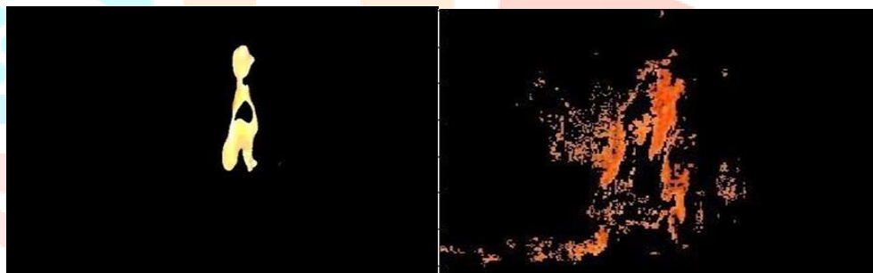
Fig 3: Output after background subtraction and color detection where fire region is detected based on the manually given threshold value of fire color.
