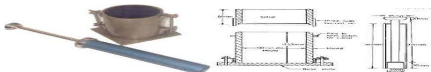
Figure 4.4 Standard Proctor test Apparatus
