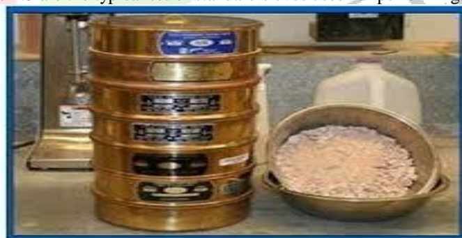
Figure 4.3 Set of Standard Sieves
