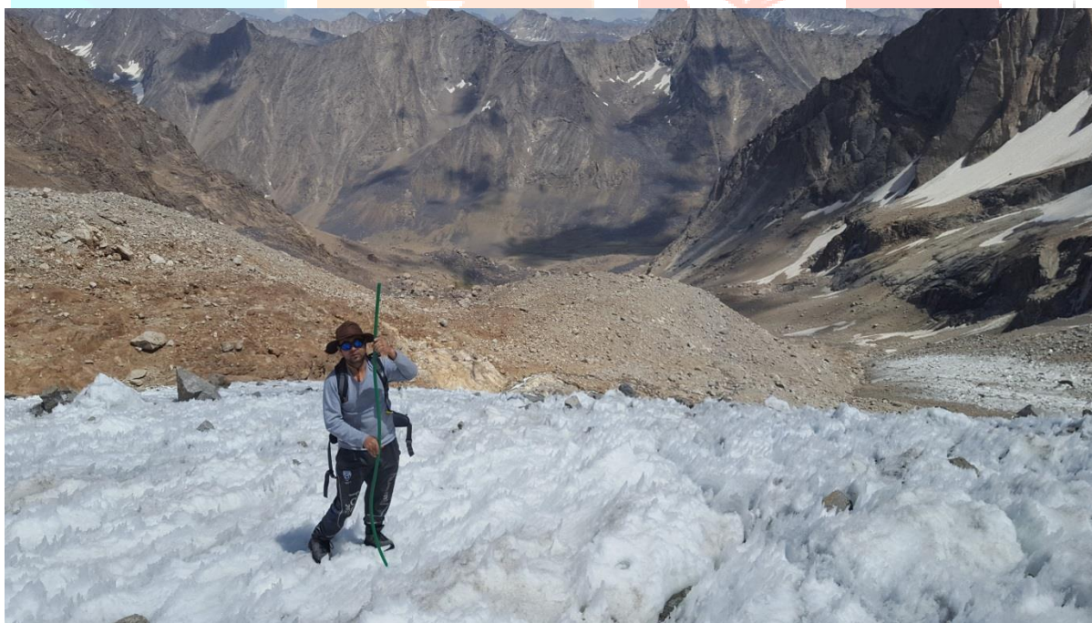
Figure 4. The image shows melting rate in PY-20 stick during one year on the ablation zone, the stick are made of PPR pipe with length of 4 meters. Photo by research team.
