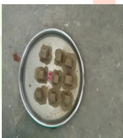
Fig.8 30% GGBS after melting
