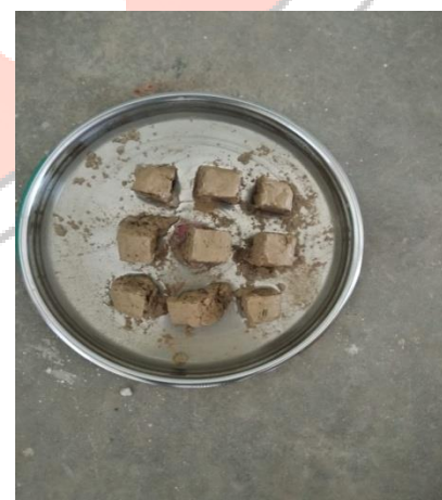
Fig.9 40% GGBS after melting
