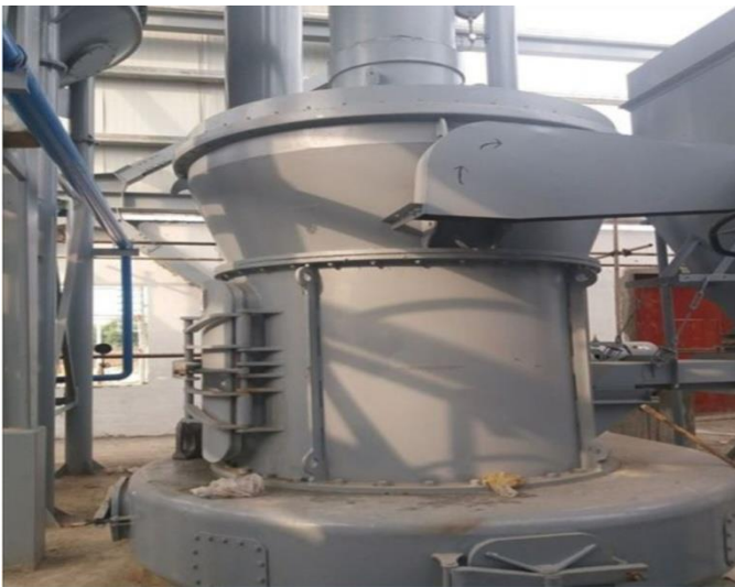
FIG.1 Crusher and binding machine for bentonite production
