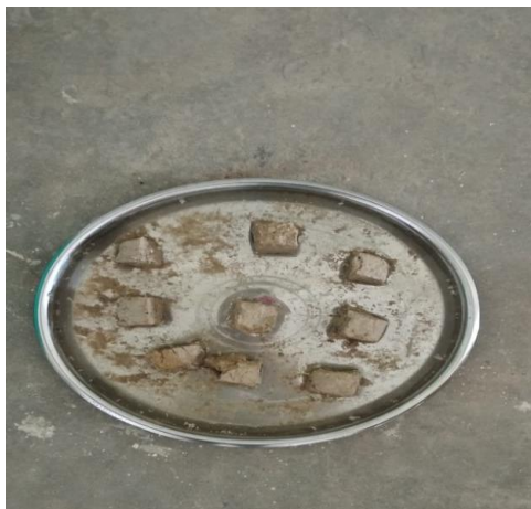
Fig.7 20% GGBS after melting
