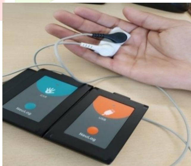
Fig. 2- Placement of GSR Electrodes on Fingers (Sharma & Kaur, 2020)
