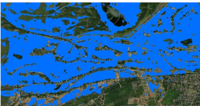
Fig 8.7: Sentinel- I SAR dual color resolution image showing flooded regions for area under consideration in Fig 8.6 in July, 2020. The black coloured regions depict the agricultural lands and other low-lying areas that get submerged under water during the monsoon.
