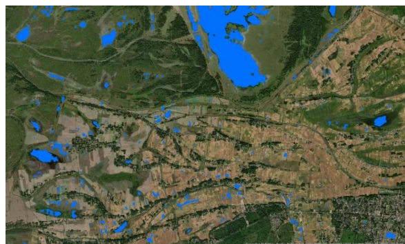
Fig 8.8: Sentinel- I SAR dual color resolution image showing area under consideration in Fig 8.6 in January, 2020. The black coloured regions depict the permanent water bodies. Since there is very little rainfall in January, most of the areas remain dry and there is no flooding.
