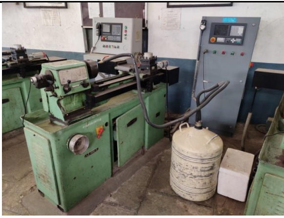
Figure 1 Cryogenic assisted retrofitted CNC
