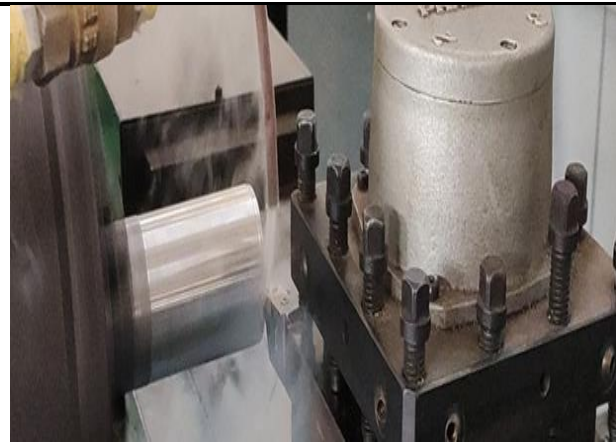
Figure 2 AISI D2 steel turning
