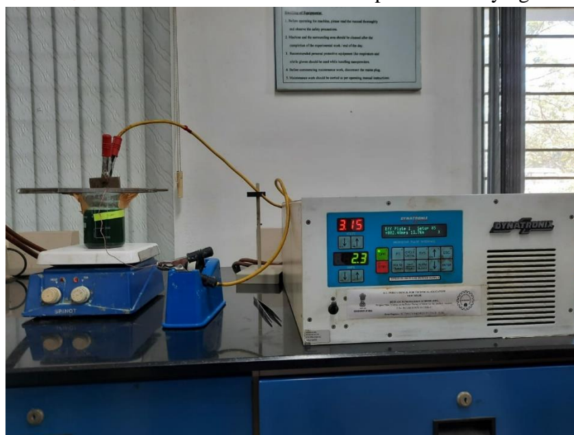
Dyanatronix Pulse Rectifier and plating setup
