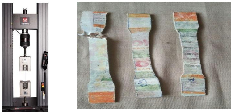
Fig. 3.1 Tensile test conducted experiments and tested samples
