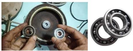
The most crucial components of every fan are its bearing and shaft, at which the fan blade is attached. The bearing is a stationary cylinder inside which the shaft rotates. Bearings in ceiling fans are pre-lubricated when they're installed.
