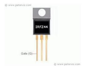
The IRFZ44N is a N-channel MOSFET with a high drain current of 49A and low Rds value of 17.5 m $\Omega$ . It also has a low threshold voltage of 4V at which the MOSFET will start conducting. Hence it is commonly used with microcontrollers to drive with 5V.
