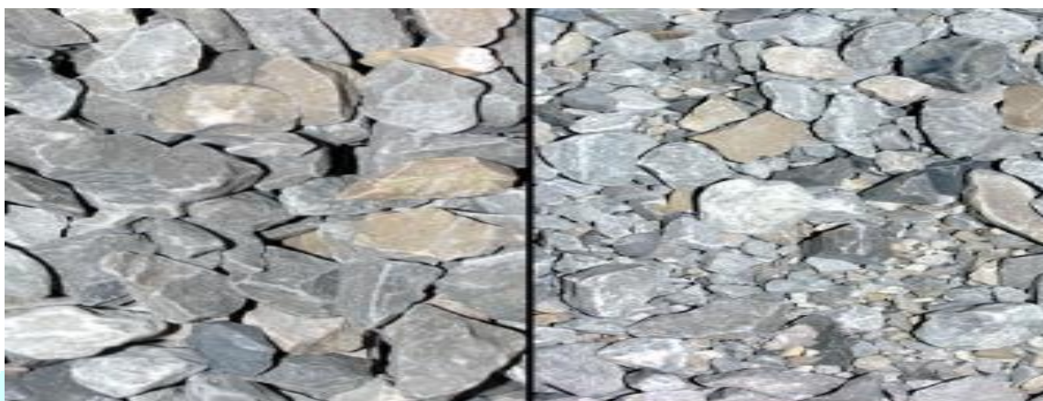
Fig. 2: Los Angeles Abrasion Test.
