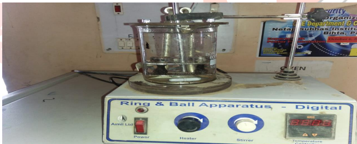
Fig. 3: Softening point test apparatus
