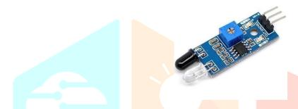
IR sensor is an electronic instrument It can be done by emitting or detecting infrared radiations. There are two types of infrared sensors active and passive. Active infrared sensors both emit and detect infrared radiation. Active IR sensors have two parts one is light emitting diode (LED) and another one is receiver. When an object comes close to the sensor infrared light from the LED reflects off of the object and is detected by the receiver.
