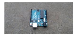
Arduino boards are able to read inputs light on a sensor, a finger on a button and turn it into an output activating a motor, turning on an LED. You can tell your board what to do by sending a set of instructions to the microcontroller on the board.
