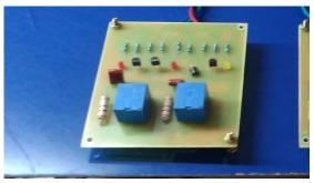
A relay is an electrically operated switch. Current flowing through the coil of the relay creates a magnetic field which attracts a lever and changes the switch contacts. The coil current can be on or off so relays have two switch positions and they are double throw (changeover) switches. Relays allow one circuit to switch a second circuit which can be completely separate from the first.
