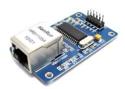
This internet module is used to connect the arduino with internet. Then the details are send to the mobile phone through this device. This device is connected with application.
