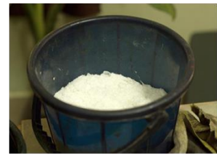
Alum is mixed with colour to strengthen the hold of colour on fabric
