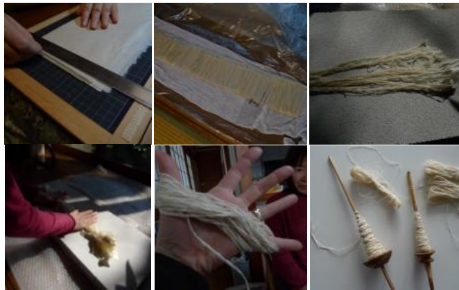
Figure 7: thread making process from recycled paper
